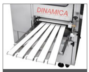
Finger belt to connect the Dinamica with a moulding station or a line (Optional).
