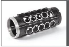
Due to the innovative design of the rounding drum, the DINAMICA, with only one drum, can cover the entire weight range in one single machine execution, and, of course, with the highest standard for rounding that only a drum system can deliver at the maximum speed of hourly production.
