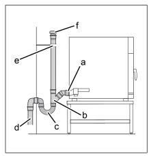
Image: Wastewater line to a permanent connection
