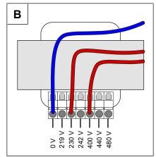
Image: A Transformer position T0, only for unit without neutral wire; B Transformer connection
