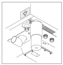
Image: Connecting the potential equalisation circuit
