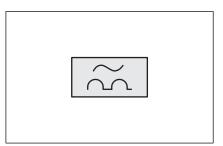
Image: RCD switch type A, circuit symbol
