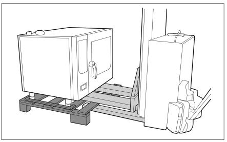
Image: Lifting the unit off the pallet
