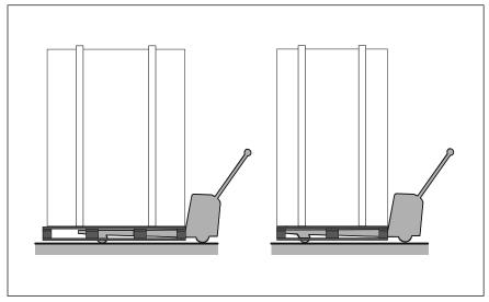
Image: Lengthwise and crosswise transport on pallet
