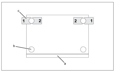
Image: Arrangement of the base plates (view from above)
