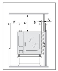
Image: Minimum clearances to walls, ceiling or units
