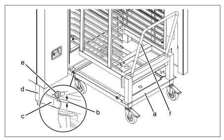
Image: Aligning the tray trolley with the insertion system
