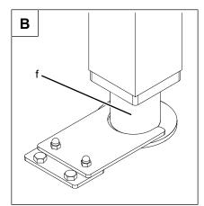
Image: A: Position of the floor plate; B: Floor plate screwed to the floor
