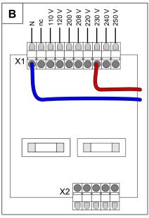
Image: A Transformer position T1; B Connection for transformer controls
