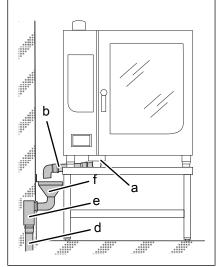
Image: Connecting a wastewater line with an unobstructed discharge
