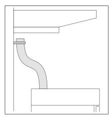
Image: Connecting the exhaust air line
