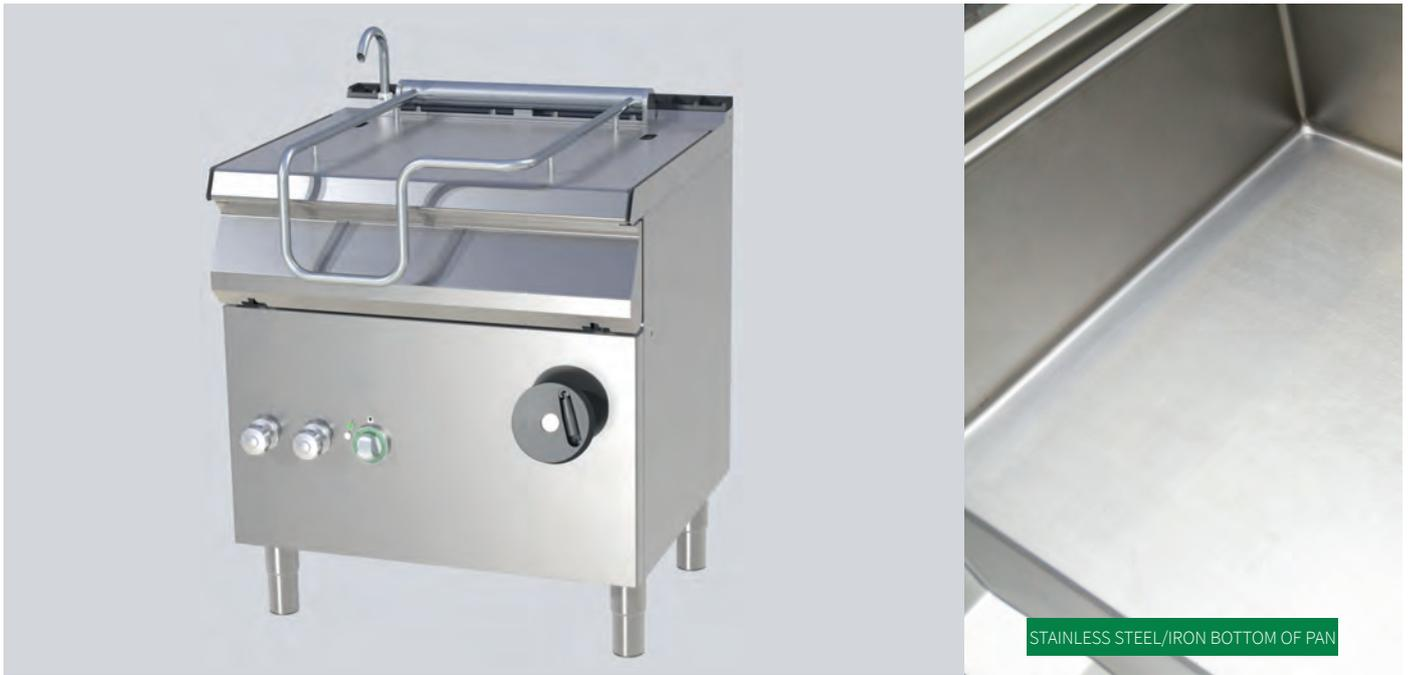
All units are made of AISI 304. Top plate thickness is 1,5 mm. Steam collector inside a lid. Water connection taps for hot and cold water. Resistance covers whole area of tank bottom, with no obstruction (the bracket of tilting system is fixed to the side part of tank). Two versions of tilting system – smooth manual operation or fully motorized tilt by a push button switch. Iron or stainless steel bottom, possibility of filling hot and cold water.
