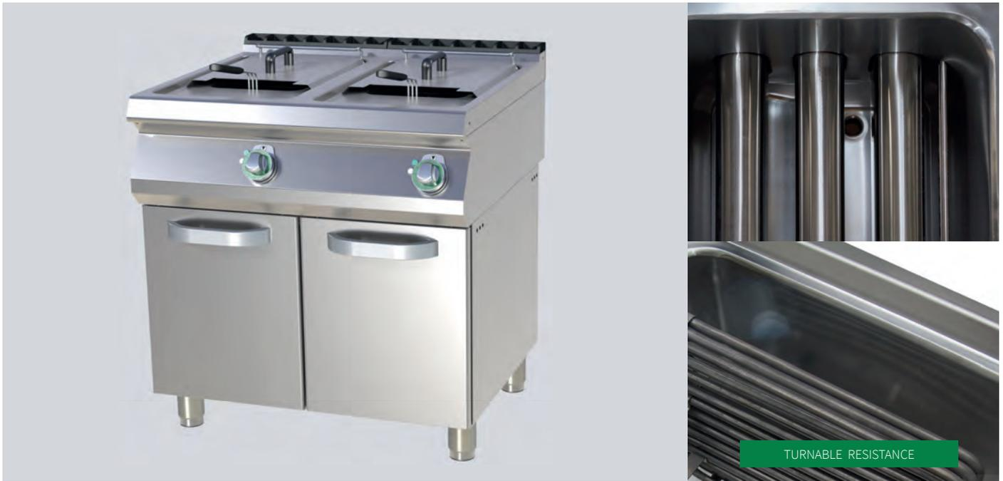
Pressed basins with ergonomic inner shapes and angles for easy cleaning and maintenance. All units are made of AISI 304. Top plate thickness is 1,5 mm. Selection of different power outputs and basin volumes. Rotating resistances with a solid support, ensuring a proper cold zone underneath. Oil drainage into the GN basin inside neutral cabinet. Standard sizes of 400 and 800 mm in width.
