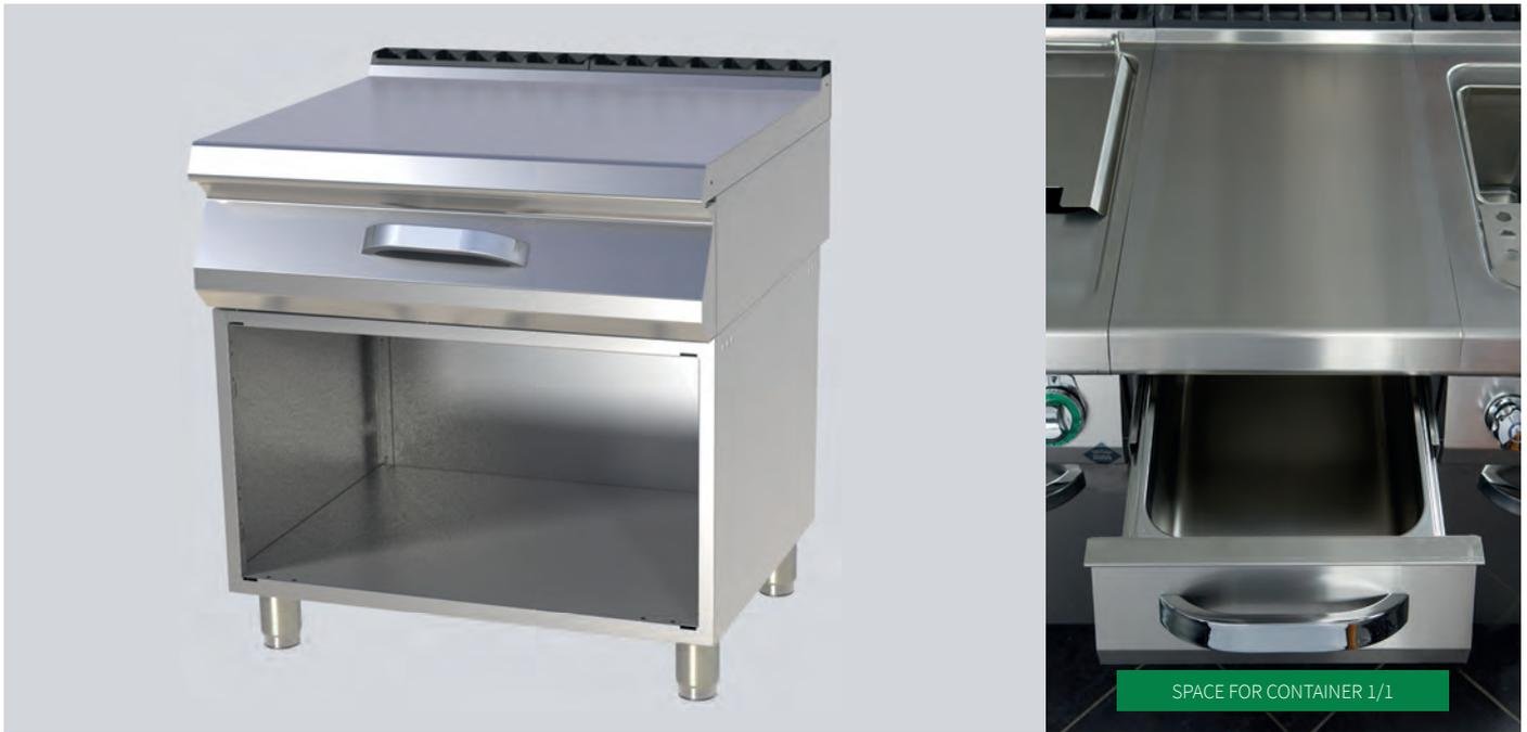
Upper plate made of AISI 304 with thickness 1,5 mm, body made of AISI 304 0,8 mm. Drawers with dimensions of GN 1/1 and 2 x GN 1/1 for ingredients or accesories.
