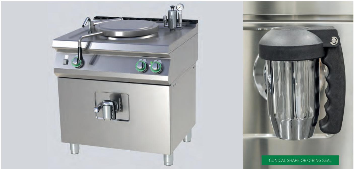
All units are made of AISI 304. Indirect heat in double-skin tank. Semi-automatic water filling system for easy and safe operation. Pressure controlled by safety valve 0,5 bars and manometer.
