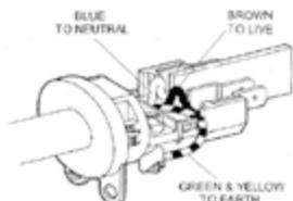
The wires in the mains lead are coloured in accordance with the following code: Green & Yellow = Earth - Blue= Neutral - Brown= Live
