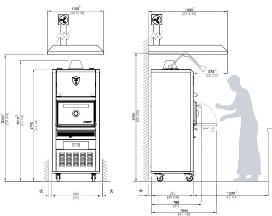
\* MINIMUM DISTANCE TO FLAMMABLE ELEMENTS: 300 mm [12 in] / RECOMMENDED DISTANCE TO ANOTHER ELEMENTS: 100 mm [4 in]
