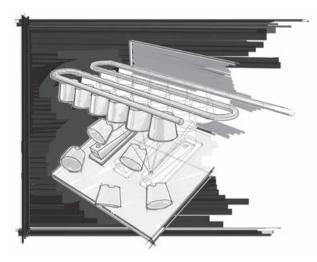
Horizontal ice evaporator and spray-system technology
