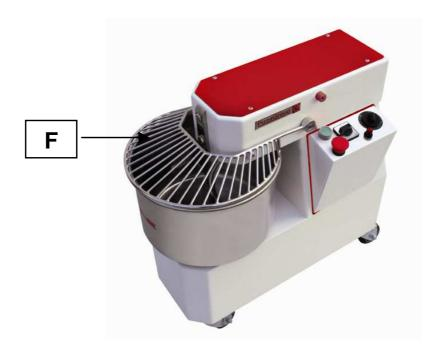
protection **F**, set the timer **C** at a defined time and press the green start button **B**.
