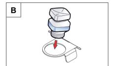
Image: A: Inserting the cartridge into the spring holder; B: Inserting the cartridge into the holder
