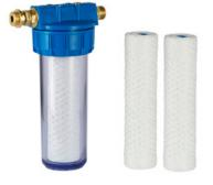
The NK filters are available in two sizes of 5" and 9" and can have two types of filtration, the first with wire-wound cartridges, the second with activated carbon cartridges, the latter for the elimination of odors or bad flavors from the water.
