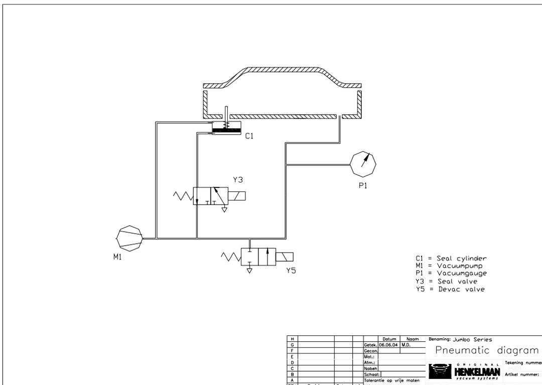
Diagrams are shown for standard configurations.
