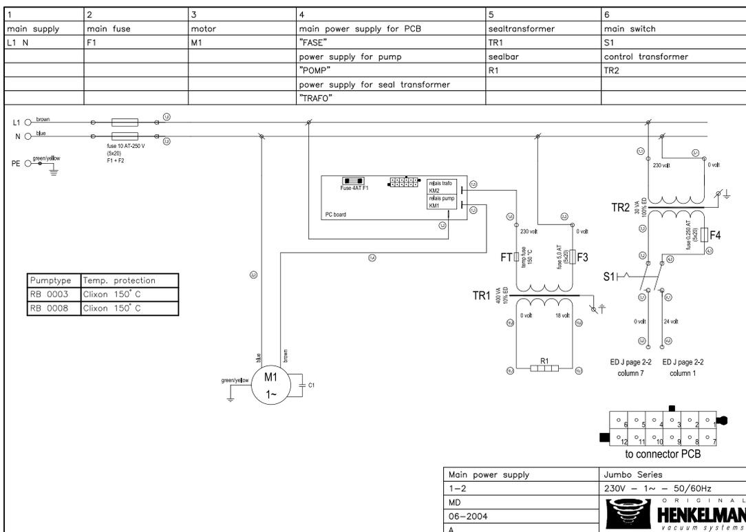
Diagrams are shown for standard configurations.
