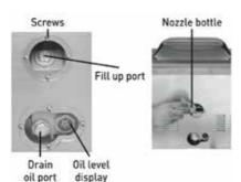
Add oil to the pump if the following situations occur. Important! Make sure the pump oil is above MIN marking and check regularly.
