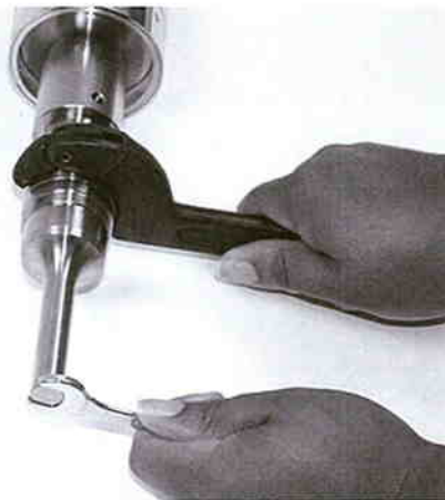
Figure 4.2 Connection or Removing Tip and Horn
