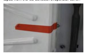
Remove first the ice deflector/evaporator cover then the masking tape from the ice thickness sensor.
