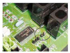
Manual reset mode and water purge out for a short time only at beginning of every harvest cycle plus a full water purge every six cycles - Recommended for normal/hard water - JUMP IN TWO contacts of J1
