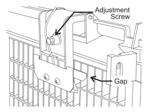
Ice Thickness Sensor Adjustment
