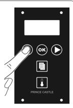
From the SET PLATEN TEMPERATURES screen, press the OK button.
