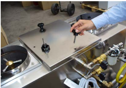
Unscrew the 4 fastening knobs clockwise to open the inspection window
